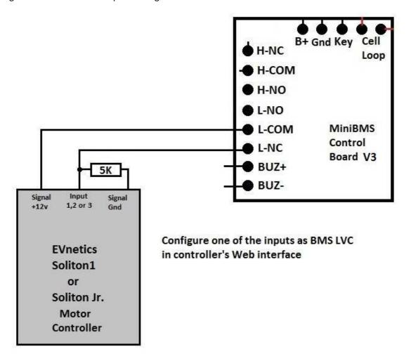
**Auxillary 12V battery note:** MiniBMS relies on constant power supplied from your 12V aux battery. Please make sure your 12V battery is properly charged at all times to ensure correct BMS operation. For safety reasons MiniBMS will shut off the charging process if it loses 12V power to the head end control board, which may leave you with undercharged pack unexpectedly.
