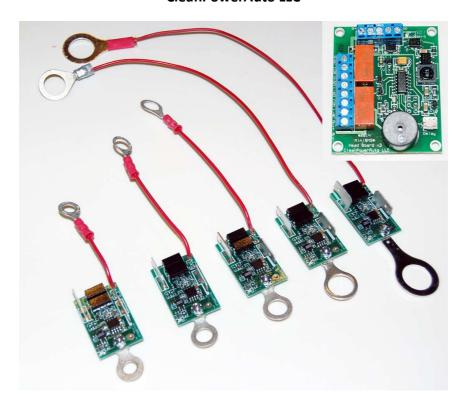
MiniBMS is a battery management system designed for LiFePo4 cells, used in Electric Vehicles. MiniBMS is designed to be reliable and cost effective solution; it has most basic functions, implemented via simple one wire opto-isolated interface called OptoLoop, which also allows easy installation and troubleshooting.
