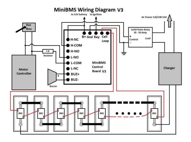
If your motor controller has separate input for BMS's LVC signal you should use it instead of cutting into throttle circuit.
